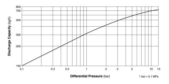
1. Differential pressure is the difference between the inlet and outlet pressure of the trap.
