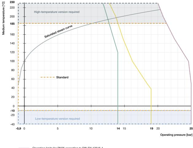
Operating limits for PN25 according to DIN EN 12516-1
